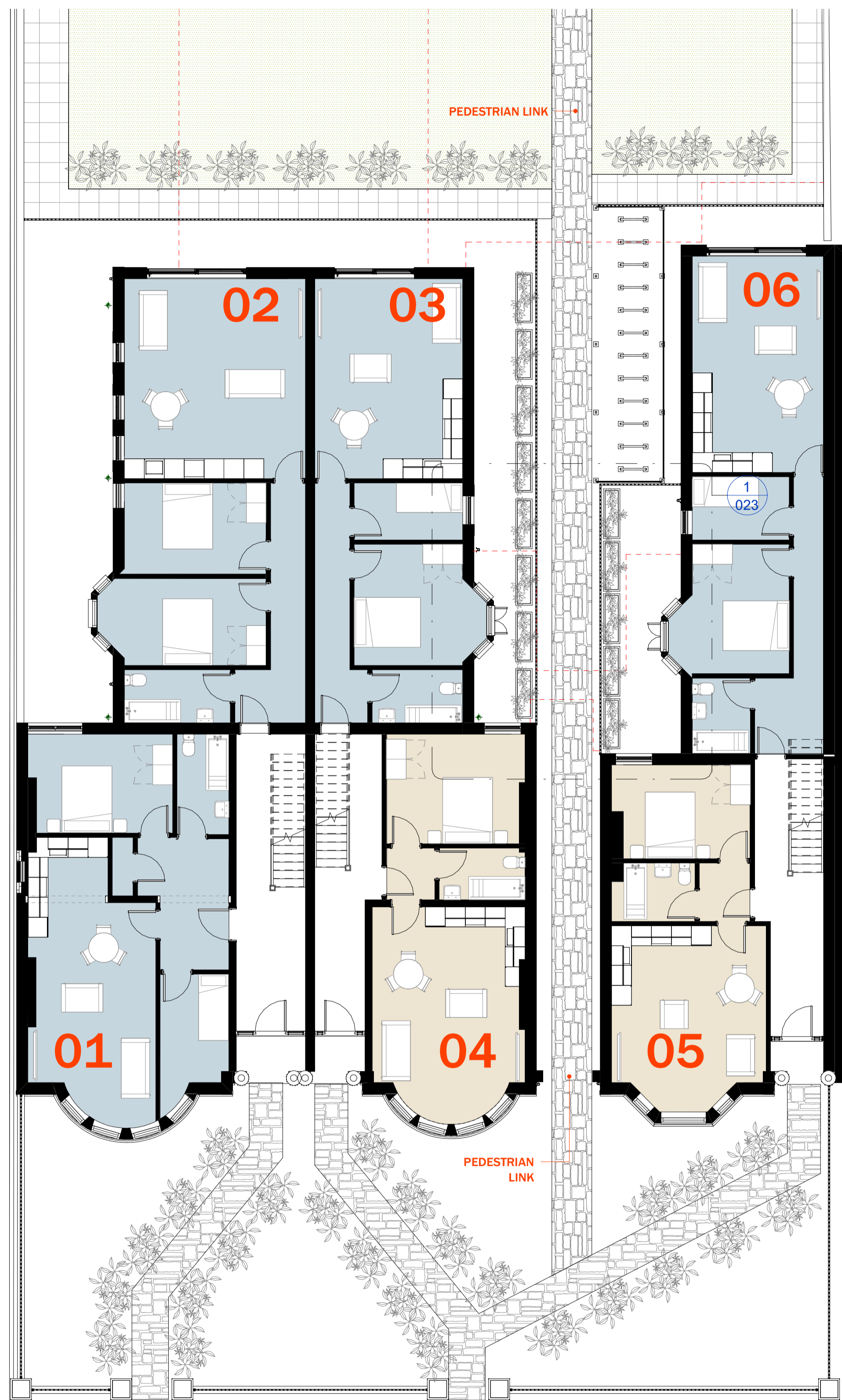
0 | PROPOSED GROUND FLOOR PLAN 1:100
